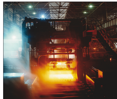
Descaling of steel sheets and profiles.
